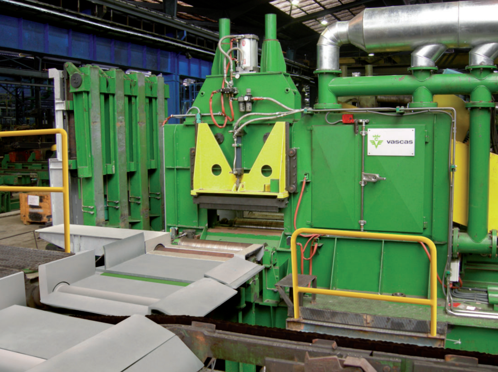
Vascas TR-2/1250 model abrasive cut-off machine for hot cutting at the end of a rolling mill
