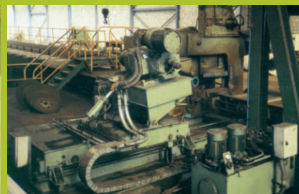
Vascas TR-2/1000 model abrasive cutting machine at the exit of a cooling bed
