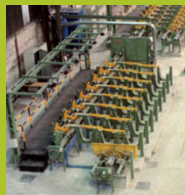
Vascas TR-1 abrasive cut-off machine in a cold finishing line
